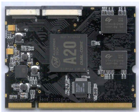
A20 Dual Core Module (Pin for Pin Compatible with A10 Single Core Module)
